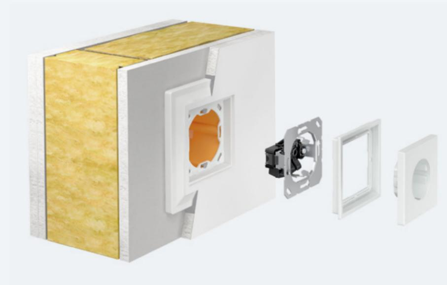
The prerequisite for dry wall mounting is the double board layer of the dry wall. The plastering adapter has the same installation height as plasterboard (12.5 mm) and enables the tight fit and firm bond with the surface.
