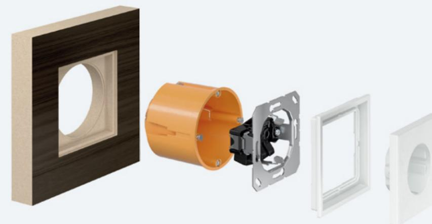
Using the drawing data specified by JUNG, the furniture builder can work to millimetre accuracy. After cutting the recess, commercially available cavity wall boxes are placed to install the desired insert, the LS ZERO frame and the cover flush-mounted.
