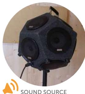
The measurement is performed by activating a specific noise source in the emitting environment and measuring the sound pressure levels in both environments (emitter and receiver). The sound reduction index is given by the difference of the two measured levels. Therefore, the higher the  $R_w$  value, the better the acoustic performance of the construction assembly.
