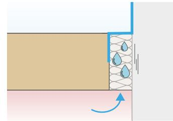
The inner protection level is not sealed, but the outer level is sealed: there is a high risk of humidity-laden internal air penetrating the joints and forming condensation in the intermediate level.
