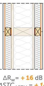
Create a self-supporting structure separated from the structure by at least 1 cm and add mass with **SILENT WALL BYTUM** or **SILENT WALL BYTUM SA** to the plasterboard sheet
