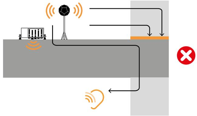
The profile, placed only above the floor, interrupts part of the propagation of vibrations generated by airborne noise. The absence of the lower profile causes part of the airborne noise and all impact noise to propagate indirectly.
