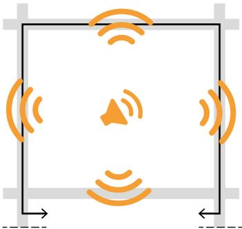
Airborne noise is transmitted to adjacent rooms either by air or by structure, following the paths represented by the arrows (lateral transmission see page 84).
