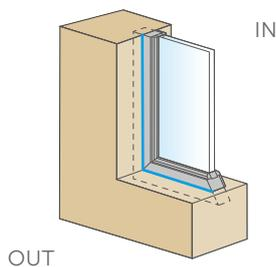
**The most external level must guarantee protection against weather.** If not properly treated, it can lead to problems of infiltration and accumulation of stagnant water at the bottom of the window hole.
