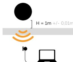
The RUBBER BALL is used to simulate "soft" and "heavy" impacts, such as a barefoot walk or a child jumping.
