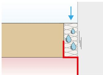
The inner protection level is sealed, the outer level is not: the joint is not effectively protected against wind and rain from outside.
