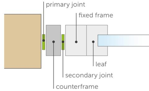
The **PRIMARY JOINT** is the first installation node between the structure and the counterframe. The **SECONDARY JOINT** is the junction between the counterframe and the frame.
