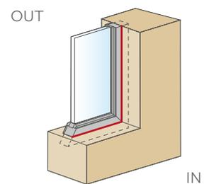
**The most internal level must be airtight.** Its function is to prevent the passage of vapour laden air, which could create condensation in the joints and mould on the surface.
