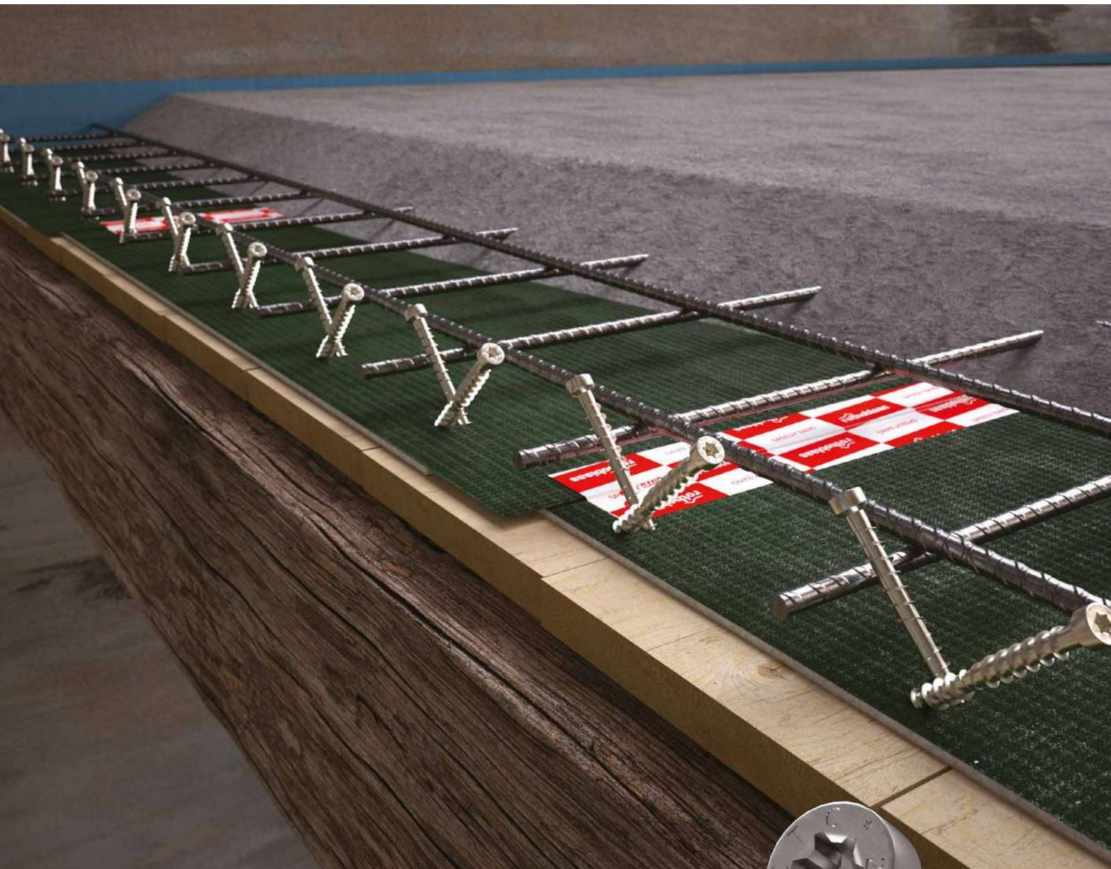
CTC is the connector for timber-to-concrete floors. CE certified, it allows to connect a 5 or 6 cm reinforced concrete slab to the timber beams of the underneath floor, obtaining a new timber-concrete structure with extraordinary strength and excellent static and acoustic performance. It is an approved self-drilling, reversible, fast and minimally invasive system.
