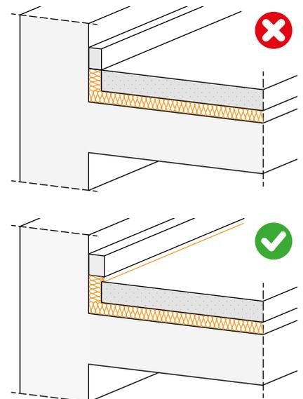
The skirting board must be installed after the SILENT EDGE has been cut, ensuring that it is always suitably raised from the floor.
