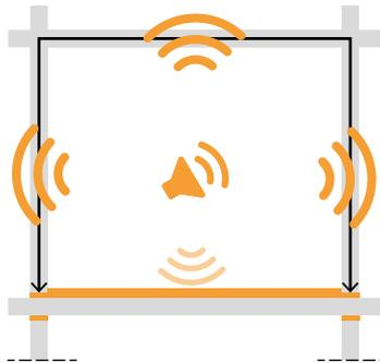
The floor assembly reduces noise propagation through the ceiling (see page 22). The use of resilient decoupling profiles reduces the propagation of airborne and structural noise (see page 86).
