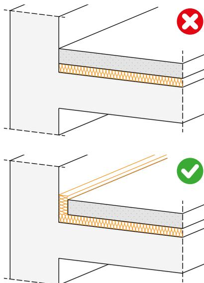
It is important to use the SILENT EDGE perimeter strip to ensure that the resilient layer is continuous around the entire perimeter of the room. The SILENT EDGE should only be trimmed after the floor has been installed and grouted.
