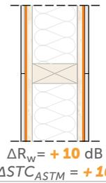
Add strips of resilient layer **PIANO A**, **SILENT FLOOR PUR** in strips and **SILENT FLOOR TEX** in strips and mass by coupling **SILENT WALL BYTUM** or **SILENT WALL BYTUM SA** to the plasterboard sheet
