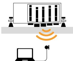
The TAPPING MACHINE is used to simulate "light" and "hard" impacts, such as walking with heeled shoes or the impact caused by falling objects.
