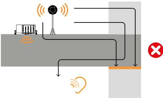
The profile placed only below the ceiling interrupts the propagation of vibrations generated by impact noise. As we can see, this configuration lacks the profile that interrupts the propagation of vibrations generated by airborne noise.
