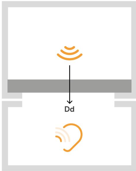
In a laboratory, the component to be tested is installed in rooms decoupled from each other that are designed specifically for that purpose. Measurements in the laboratory are characterised by direct transmission, i.e. only through the separating construction element.
