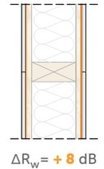
Add a resilient layer **SILENT FLOOR PUR** or **SILENT FLOOR TEX** between the base structure and the plasterboard sheet
