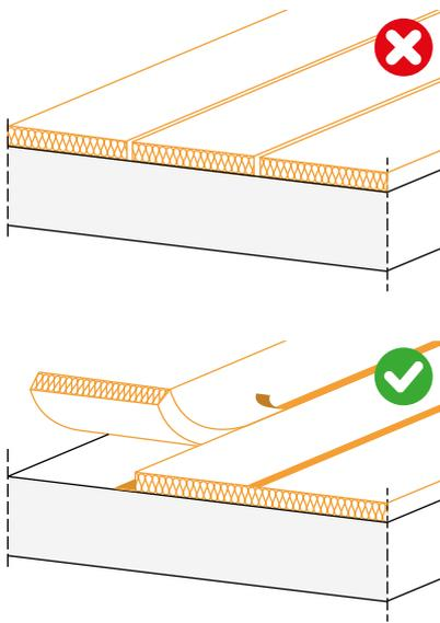
The resilient layer must be continuous because any gap would represent an acoustic bridge. When installing underscreed mats, care must be taken not to create discontinuities.
