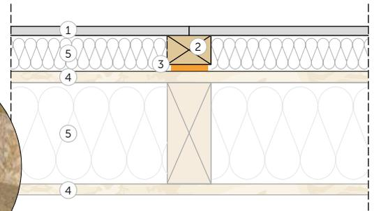
Add the supporting wall to the base frame and decouple it using strips of SILENT FLOOR PUR.
