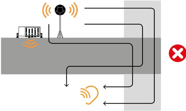
If resilient profiles are not included in the design, the propagation of vibrations at the structural level is not interrupted and the contribution of flanking sound transmission can be significant, both for airborne sound and the impact sound.
