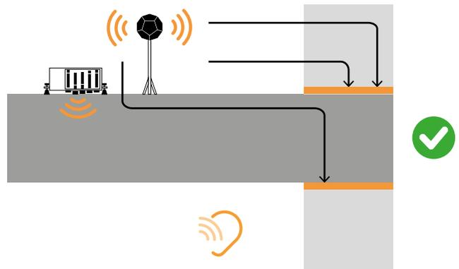
Due to the presence of the resilient profile both above and below the floor, all lateral transmission paths were interrupted and the propagation of vibrations through the structure was minimised.
