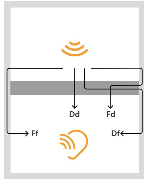
When the sound reduction index is measured on site, the value is lower than that measured in the laboratory for the same construction assembly. This is because transmission between rooms is also characterised by flanking sound transmission, i.e. the contributions to propagation made by structural or rigid building elements.
