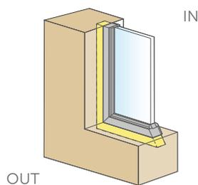
**The intermediate level must guarantee thermal-acoustic performance and mechanical fixing.** When choosing products, bear in mind that a good anti-noise solution is not always thermally effective.
