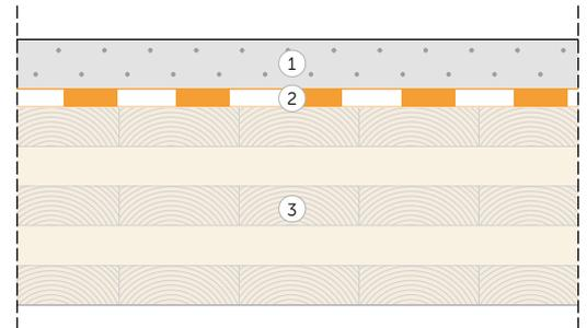
Thanks to the addition of the floating screed system on the raw CLT.
